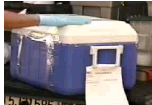
Cooler lid secured with shipping tape around each end.
